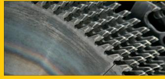
Final result following immersion process using ultrasonic vibrator and surface agitation (about 20–60 minutes without the need for any extra mechanical work such as brushing, etc., using a cleaning solution in a 1% concentration).
